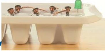
Do you know what a voltaic battery is? You probably do! Voltaic batteries come in all shapes and sizes, turning chemical energy into the electrical energy we need to power our cell phones, iPods, tablets, cars... you name it! These batteries seem pretty complicated, but you can make a real voltaic battery right at home! Grab some vinegar, nails, copper wire, and an ice tray... you're in for a lesson in circuits you'll never forget.
